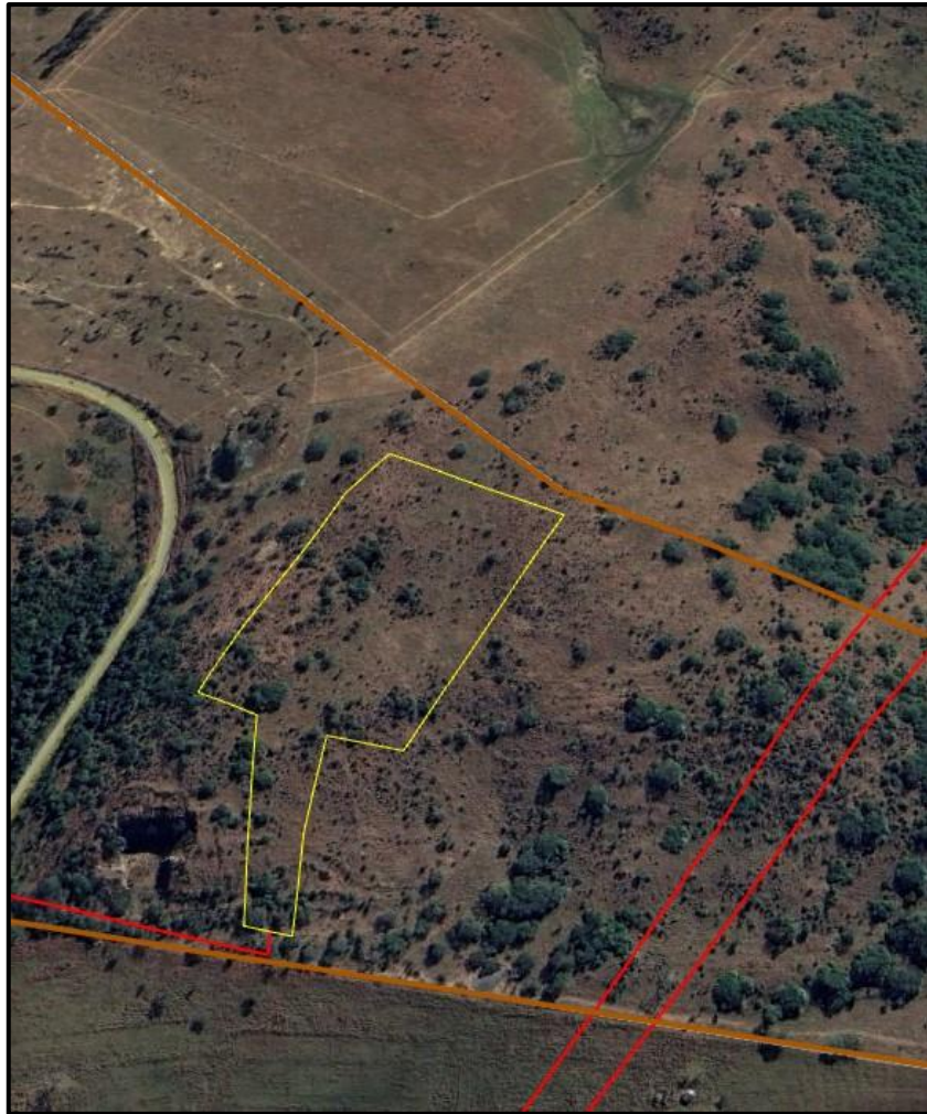
Figure 4: All stockpiles within the proposed mining area will be >200 m from the adjacent power lines (red lines) (image obtained from Google Earth).
